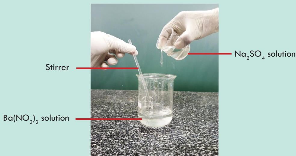
Figure 1.6 Double displacement reaction between \text{Na}_2\text{SO}_4 and \text{Ba}(\text{NO}_3)_2
